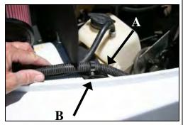
**12.** A) Using a <sup>1</sup>/<sub>4</sub>"-20 bolt, washers, and nut, bolt the **CAD** to the fender. B) Install the wire loom clamp into the hole in the **CAD**, as shown.
