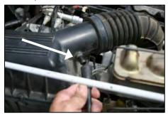
2. Unhook vacuum line from airbox, and remove from vehicle at the canister below the master cylinder. (Save for later use.)
