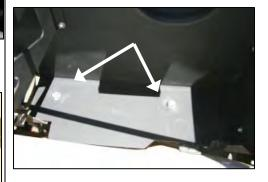
**10.** Install two ¼"-20 bolts and washers thru the top, and fender washers and nuts on the bottom, where the factory grommets were removed.
