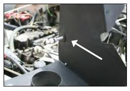
9. Carefully slide the CAD over the support rod, and then slide the supplied grommet over the rod, and into the hole in the CAD as shown. Rotate the CAD and place into position on the factory airbox mount. Reinstall the radiator support rod, and tighten the nut.
