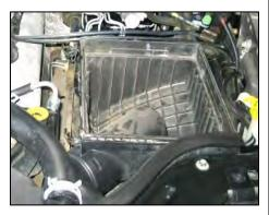
2. Remove the factory air filter box lid, accordion tube, and air filter. (<u>Note</u>: leave factory air filter base installed in vehicle)
