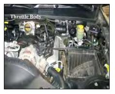
5. Remove the factory air box silencer coupler from the throttle body.
