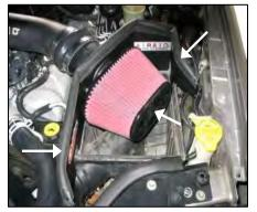
**11.** Mount the Airaid Premium filter & weather strip onto the
