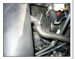
**10.** Connect the factory breather hose to the Modular Intake Tube & secure hose with the
