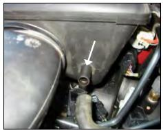
**3.** Disconnect the breather hose from the factory air box silencer.
