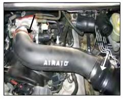
**9.** Position the Modular Intake Tube assembly to connect the reducer to the throttle body and the hump hose to the Airaid Cool Air Dam. (*Note: leave the hose clamps loose until final assembly*)
