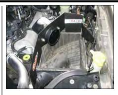
7. Position the Airaid Cool Air Dam in place of the factory air box and snap into place.
