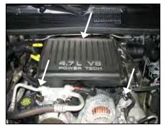
4. Loosen the hose clamp on the throttle body & both 10mm bolts securing factory air box silencer to intake manifold. Remove the factory air box silencer from engine compartment.
