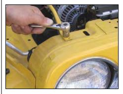
**9.** Using a 13mm socket, remove the radiator rod support bolt on the passenger side. Retain bolt for later use.
