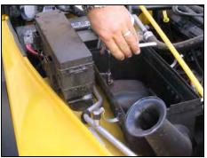
5. Using a 5/16" socket, remove the three nuts and bolts mounting the factory air filter housing to inner fender. Remove air filter housing.
