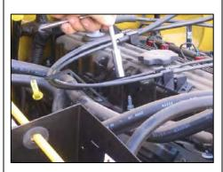
**16.** Remove one valve cover bolt on the passenger side nearest to the oil fill cap. Use this bolt to mount the supplied mounting bracket to the engine as shown above. Leave bolt loose until final assembly.
