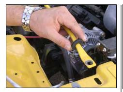
**11.** Using the supplied thin grommet, position it over the passenger side radiator support rod as shown above.
