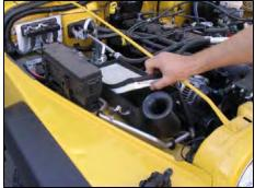
**4.** Remove factory air filter from air box.
