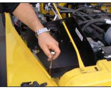
14. Using the supplied ¼ x 20 nut, bolt and washers, mount the front of the Airaid Cool Air Dam to the inner fender.
