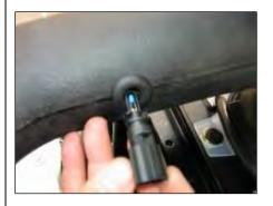
**18.** <u>For 2005-06 Vehicles:</u> Install the supplied rubber grommet with the hole. Next, install the factory air temp sensor retained from step 3 into the grommet.
