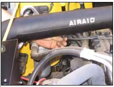
**23.** Mount the Airaid intake tube to the valve cover bracket using the supplied <sup>1</sup>/4" bolt and washer as shown above.
