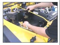
**12.** Carefully slide the Airaid Cool Air Dam assembly over the passenger side radiator support rod. Be careful not to scratch the paint. Insert the rubber grommet into the panel for final positioning of the assembly.
