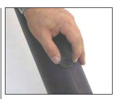
**17.** For 1997-2004 vehicles only: Install the supplied rubber grommet with out the hole into the Airaid intake tube.
