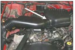
1. <u>Disconnect the negative battery cable.</u> Loosen the hose clamp that holds the factory intake tube to the resonator.
