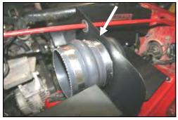
**16.** Install the urethane hump hose (#5) onto the back side of the **CAD** tube using two #72 hose clamps (#17). Tighten <u>only</u> the hose clamp on the metal tube for now.
