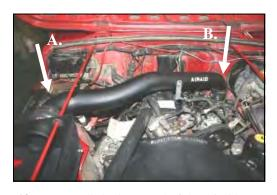
19. A.) Install the large end of the Airaid Intake Tube into the hump hose.B.) Now slide the small end into the reducer on the throttle body.
