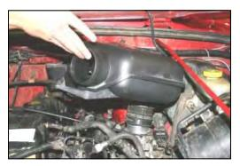
**6.** Remove the resonator from the vehicle.
