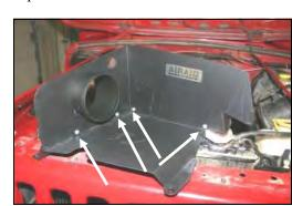
**11.** Assemble the two Cool Air **D**am panels (#2) & (#3) using the four 6-32 screws (#8), #6 flat washers (#9), and nuts (#10), as shown.
