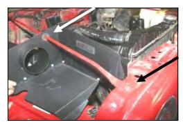
**13.** Align the **CAD** over the mounting holes, and re-install the factory bolt from step #10 in the radiator support. Slide the grommet forward into the hole in the **CAD** as shown.
