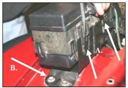
**8.** A.) On the right fender, pry two tabs away from the fuse box, lift it up and set it off to the side. B.) Next, remove and save the outside bolt from the fuse box mount. It will be re-used in step #14.
