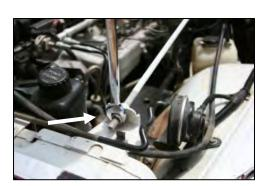
**8.** Using a 9/16" wrench, loosen the nut on the radiator support rod, and lift it up out of the slot.
