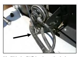
**11.** Slide the **CAD** bracket under the horn mount and reinstall the factory bolt from step 5.
