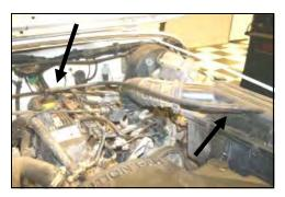
**1.** <u>Disconnect the negative battery cable.</u> Remove the factory valve cover breather hose from the airbox, and the valve cover.
