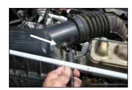
**2.** Disconnect the vacuum line from the airbox and at the canister below the master cylinder. (Save for reuse.)
