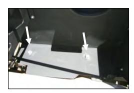
10. Install two  $\frac{1}{4}$  - 20 x 5/8" hex bolts (#13) and 1/4" flat washers (#14) thru the top of the **CAD**, and fender washers (#15) and locknuts (#16) on the bottom, where the factory grommets were removed.
