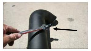
**14.** Install the ¼" barbed fitting (#22) into the intake tube.
