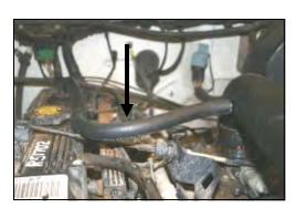
17. Replace the factory breather hose with the ½"x 14" breather hose (#8) between the valve cover and the intake tube using two #16 speed clamps (#21) as shown.
