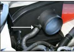
13. Install the Quick Fit assembly in the bottom of the stock air box by sliding the four tabs on the back into the slots on the airbox, once installed, re-hook the two latches. Next, install the speed clamp over the breather hose and connect it to the Quick Fit assembly as shown.
