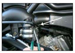
8. Carefully pull the resonator towards you and rotate the bottom up to gain access to the tie wrap holding the breather hose to the rubber coupler. Cut the tie wrap and discard.
