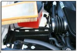
**4.** Remove factory air filter from air cleaner box.
