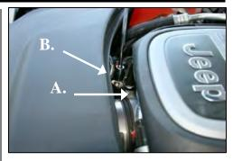
A.) Loosen the hose clamp on the throttle body. B.) With a 10mm socket, remove the bolt next to the throttle body that holds the intake resonator in place.
