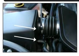
Disconnect the negative battery cable. Loosen the hose clamp on air cleaner box lid. Twist and remove breather hose from air cleaner box lid.
