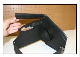
**12.** Install the weather strip on the top of the Quick Fit assembly. (*Hint: start at one end, and go towards the other end, don't start in the middle.*)
