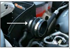
14. Install the hump hose and two #60 hose clamps on the Quick Fit assembly. Do not tighten the clamps at this time.
