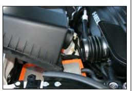
**3.** Remove the air cleaner box lid by sliding it forward, and then up, and out of the factory intake tube.
