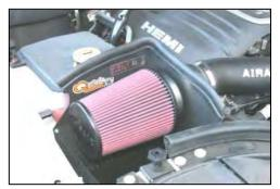
**19.** Install the Airaid Premium Filter (#1) on the Quick Fit assembly as shown, and tighten the hose clamp.
