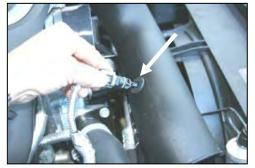
**17.** Carefully install the factory temperature sensor into the grommet. Make sure it is seated all the way in.
