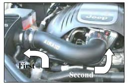
**18.** Carefully install the end of the Airaid Intake Tube (#4) into the hump hose, and then into the reducer on the throttle body as shown. Adjust the tube as needed, and then **tighten the four hose clamps.**
