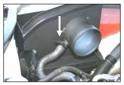
13. Install the Quick Fit assembly in the bottom of the stock air box by sliding the four tabs on the back into the slots on the airbox, once installed, re-hook the two latches. Next, install the speed clamp (#10) over the breather hose and connect it to the Quick Fit assembly as shown.
