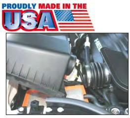
**3.** Remove the air cleaner box lid by sliding it forward, and then up, and out of the factory intake tube.
