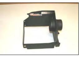
11. Assemble the two pieces of the Quick Fit panels as shown (#2&#3), using the four 6-32 screws (#12), washers (#13), and nuts (#14), that are provided in the kit.
