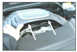
6. Carefully lift up on the engine cover *(it is held in place by grommets, no bolts)* to access the hose clamp on the throttle body, and 10mm bolt next to the throttle body.
