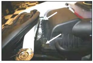
**2.** Unlatch the two clips on the factory air cleaner box lid.
