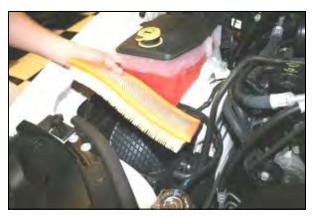
**5.** Remove the factory air filter.
