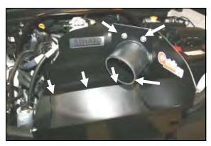
11. Install the Quick Fit panels into the factory lower airbox by lining up the three tabs in the rear of the panel, the latch holes in the front, and then re-latching the factory airbox clips. Next, using the 1/4-20x1/2" button head screws (#10) and 1/4" flat washers (#11), install the air filter adapter into the Quick Fit Panel.
