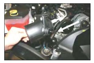
**10.** Install the  $90^{\circ}$  nylon fitting (#9), into the air filter adapter.
