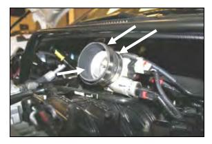
12. Install the provided reducer (#3) onto the throttle body with the smaller diameter towards the throttle body. Place the #48 hose clamp (#6) on the smaller diameter section of the reducer (throttle body side). Place the #52 hose clamp (#7) on the larger diameter side of the reducer. Leave the clamps loose for now.
