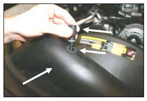
**15.** Install the rubber grommet (#12) into the Modular Intake Tube (#5). Next, slide the factory intake air temp sensor into the grommet in the tube. Make sure it is seated all of the way in.
