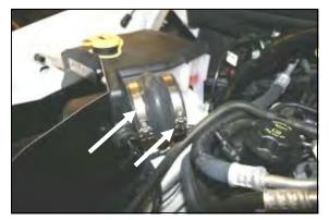
13. Install the provided hump hose (#7) onto the air filter adapter. Place a #56 hose clamp (#15) on each side of the hump hose. Tighten only the clamp on the air filter adapter. Leave the other clamp loose for now.
