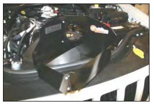
**9.** Assemble the Quick Fit panels as shown, using five 6-32 screws (#16), #6 washers (#17), and keps nuts (#18).
