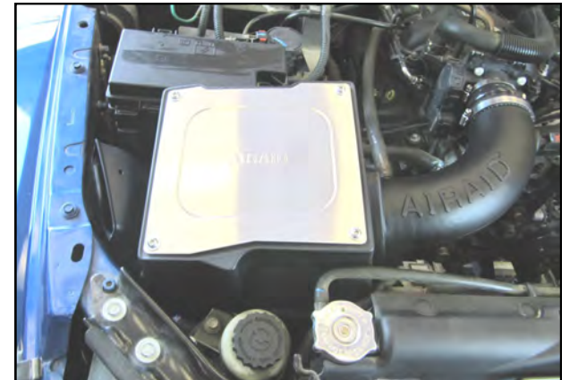
18. Double check your work! Make sure there is no foreign material in the intake path. Make sure all clamps, hoses, bolts, and screws are tight. Double check the hood clearance!
