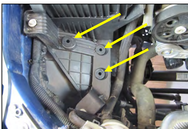
7. Replace the factory airbox grommets in the inner fender area with the three 3/8" Well Nuts (#15).
