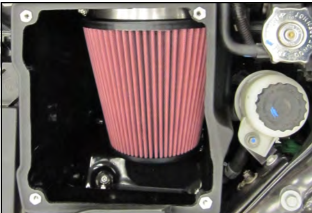
16. Slide the Airaid Synthamax Filter onto the Intake tube inside the Cold Air box and tighten the clamp.
