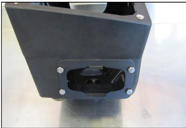
4. Install the Air Scoop Bracket (#4) into the Cold Air Box as shown by using four 1/4-20 x 5/8 Hex Bolts (#11), 1/4" Flat Washers (#12), and 1/4" Nylock Nuts (#13).
