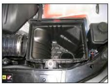
**3.** Remove the factory air box lid and flat panel filter. (*Note: Retain the factory air box base.*)
