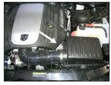
1. Loosen the hose clamp on the intake tube.
