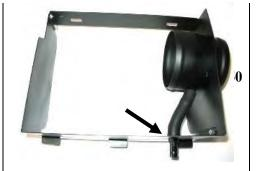
4. Install the supplied ½" hose on the Airaid CAD nipple.
