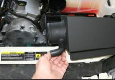
**6.** Slide the 1/2" rubber hose elbow onto the breather fitting on the side of the Cool Air Dam. Install the 2 speed clamps over the elbow, but do not tighten at this time.
