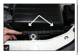
3. Unsnap the factory airbox lid by pulling the tabs towards the front of the car, then lift the lid up and slide it forward, and remove it from the bottom of the airbox.
