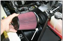
8. Slide the Airaid Premium Filter onto the filter adapter and tighten the clamp. Next, make sure the intake tube is slid all of the way on the CAD, and tighten the hose clamp. Tighten the two speed clamps on each end of the breather hose.
