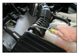
**2.** Loosen the hose clamp on the factory intake tube at the air filter lid cover.
