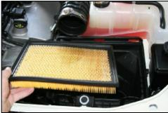
**4.** Remove factory air filter from bottom of factory airbox.
