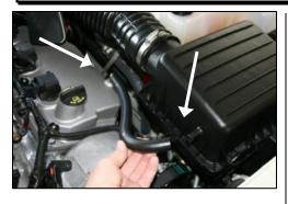
1. Disconnect the negative battery cable. Remove the breather hose from the factory air box lid and valve cover.
