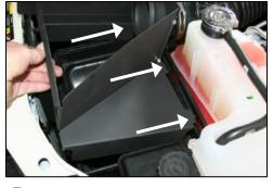
7. Slide the three tabs on the back of the CAD, into the stock airbox. (Make sure the breather hose slides onto the nipple on the valve cover.) Next push the front of the CAD down until the locking tabs snap into place.
