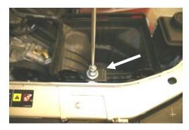
**6.** With a 10mm socket, remove and save the bolt that holds the factory air filter base to the radiator support. Remove the air filter base from the vehicle.
