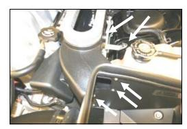
**12.** Install the hood scoop into the **CAD** using three 8-32 button head screws (#14), and three #8 flat washers (#15), leave loose. Install the L-bracket (#23) over the stud on the fender, and bolt it to the hood scoop using one 1/4-20 button head bolt (#12), and 1/4" flat washer (#13). Replace the factory nut on the stud, adjust for fit, and tighten all bolts, nuts, and screws.
