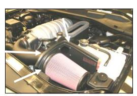
**17.** Install the Airaid Premium Filter (#1), onto the filter adapter inside of the CAD, and tighten the hose clamp. Next install the weather strip (#9) onto the top of the CAD.
