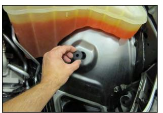
**7.** Place the 3/8 " Well Nut into the hole in the inner fender. It will be fully secured later in step **9**.
