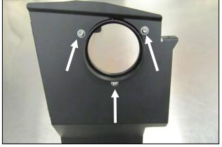
**5.** Install the Filter Adapter (#6) onto the Front Panel as shown using three 1/4-20 Button Head Screws (#12) and 1/4" Flat Washers (#13).
