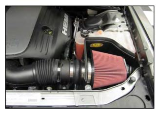
17. Install the Weatherstrip (#8) onto the top edge of the Panels with the contour rolling away from the Filter area. Complete the installation by attaching the Airaid Premium Filter (#1) to the Filter Adapter.
