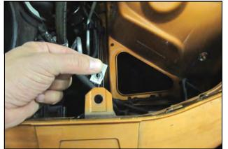
**3.** Carefully remove the speed clip from the core support tab and set it aside. It will not be reused.
