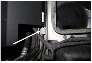
10. Snap the Line Holder (#22) onto the ABS line closest to the panel assembly and remove the adhesive backing. Gently push the Panel away from the line and slide the Line Holder behind the Panel. Relax the Panel, and allow the Adhesive pad to bond the Panel. This will isolate the Panel and prevent contact with the ABS line.
