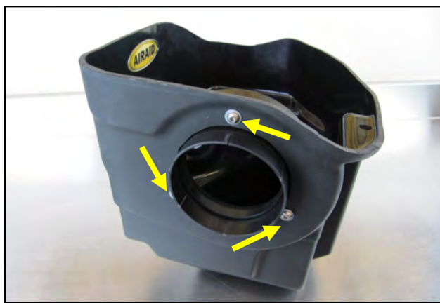
4. Install the Filter Adapter onto the Cool Air Box using the three 1/4" Button Head Screws and 1/4" Flat Washers, (#s 8&9).
