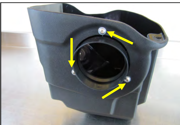
5. Install the Filter Adapter onto the Cool Air Box using the three 1/4" Button Head Screws and 1/4" Flat Washers, (#s 8&9).
