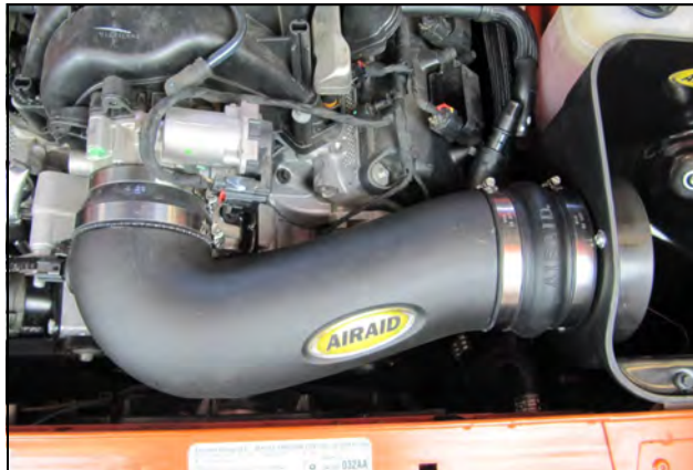
13. Insert the Intake Tube assembly into the Hump Hose first, then into the Coupler onto the throttle body. Tighten all four Clamps at this time,
