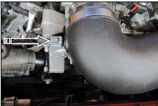
14. Reconnect the air temperature sensor.
