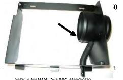
Assemble Airaid **CAD** panels using supplied hardware. Install supplied ½" nylon union through the panel hole into the ½" hose.
