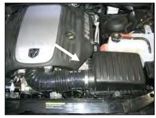
1. Loosen the hose clamp on the intake tube.
