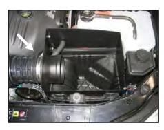
5. Install the Airaid CAD in place of the factory air box lid. Tighten factory hose clamp.
