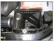
**3.** Remove the factory air box lid and flat panel filter.
