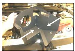
**7.** Assemble the Airaid Cool Air Dam (CAD) panels (#2, #3) using four 6-32 x 5/16" screws (#16), #6 flat washers (#17), and 6-32 keps nuts (#18).
