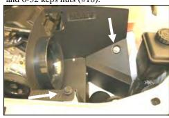
10. Install the assembled Cool Air Dam into the vehicle. Re-install the factory bolt removed in step #6 thru the CAD and into the radiator support. Next install the 3/8-16 x1" button head bolt (#10) and 3/8" flat washer (#11) thru the CAD and into the well nut. Tighten both bolts.
