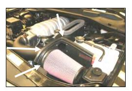
**17.** Install the Airaid Premium Filter (#1), onto the filter adapter inside of the **CAD**, and tighten the hose clamp. Next install the weather strip (#9) onto the top of the **CAD**.
