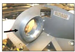
**8.** Next install the filter adapter (#6) using three <sup>1</sup>/<sub>4</sub> - 20 button head bolts (#12), and <sup>1</sup>/<sub>4</sub>" flat washers (#13).
