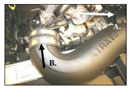
**13. A.** Install the urethane hump hose (#7) on the filter adapter using two #72 hose clamps (#20), (*Leave loose for now*). **B.** Install the reducing coupler (#8) large end on the Airaid Intake Tube (#4), using two #52 hose clamps (#19). Tighten *only* the hose clamp on the tube.
