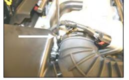
**1.** <u>Disconnect the negative battery cable.</u> Loosen the hose clamp that holds the factory intake tube to the throttle body.
