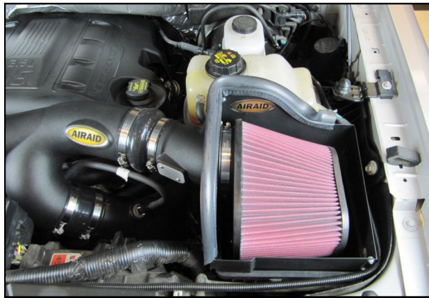
13. Install the Airaid Premium Filter onto the Sensor Tube and tighten the clamp.
