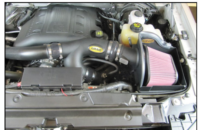
14. Double check your work. Make sure there is no foreign material in the intake path. Make sure all clamps, hoses, bolts, and screws are tight. Double check the hood clearance. Reconnect the negative battery cable.
