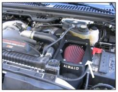
**16.** Install the black panel onto the top of the airbox using the 5 supplied stainless steel ¼" x 20 Allen bolts and washers.
