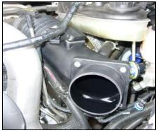
10. Slide the Airaid filter tube into factory flexible turbo inlet hose. (Note: Do not tighten hose clamp until assembly is complete.) Reconnect the sensor to the factory plug. (Either the temperature sensor or the mass air sensor, which ever you have.)
