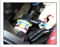
4. Disconnect electronic filter restriction gauge connector and remove the restriction gauge, and rubber grommet.(Note: retain these parts for later use.) Remove air filter inlet tube and hose assembly. USE CAUTION when removing these elements, as it is a tight fit. Be careful not to tear the factory insulation around the radiator support.
