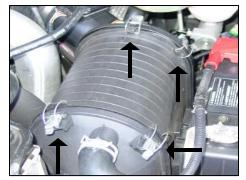
1. Disconnect negative battery cables. Disconnect and remove all four factory clips on the factory airbox.
