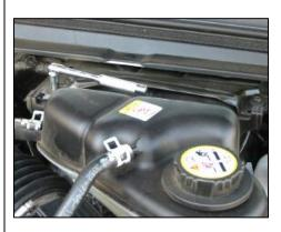
**14.** Factory tolerances may vary between the mass air sensor and the coolant reservoir,. Therefore, *it may be necessary* to loosen the two 5/16" bolts and adjust the reservoir for better clearance.
