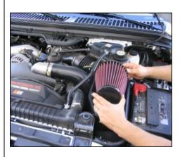
**15.** Install the Airaid Premium Filter onto the air filter adapter inside of the airbox, and tighten the hose clamp.
