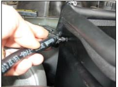
**18.** Spread the supplied hose mount over the radiator overflow hose and insert thru the hole in the side of the panel.
