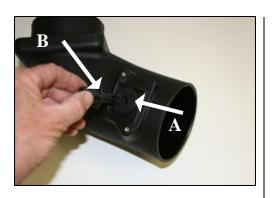
8. A.) If you have the temperature sensor shown in step #5, install the supplied grommet as shown above. B.) Install the factory air temperature sensor as shown, and then the factory grommet and filter restriction gauge. Skip to step #10.
