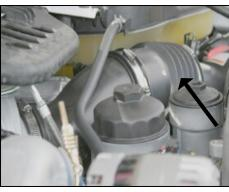
**13.** Tighten the hose clamp on the flexible turbo inlet tube.
