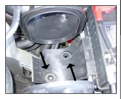
3. The filter is held in place by two rubber grommets on the bottom.(*Note: make sure factory grommets remain in lower air box support.*)
