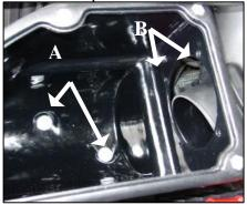
**12.** *A.*) Insert the supplied aluminum pins thru the airbox into the factory grommets. *B.*) Using 4 supplied stainless steel ¼" x 20 Allen bolts and washers, mount the air filter tube to the airbox.
