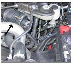
7. Remove complete factory air filter tube assembly. (Note: do not remove flexible turbo inlet hose from turbo housing.)
