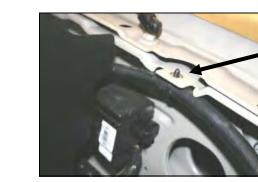
**18.** Slip the black plastic hose mount (#26) over the radiator overflow hose. Next, place one <sup>1</sup>/<sub>4</sub>" flat washer (#15) over the hole on the inner drivers side fender. Slide the hose mount prongs thru the fender and thru the washer.
