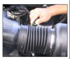
**14.** Disconnect valve cover breather hose from factory intake tube and valve cover.
