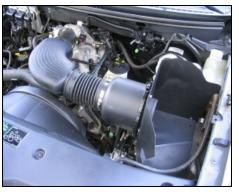
**8.** Install the Airaid Cool Air Dam assembly on vehicle using the factory intake tube clamp.
