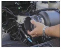
17. Install the supplied silicone hump hose and two #72 hose clamps on factory air filter assembly. Leave hose clamps loose until final assembly.
