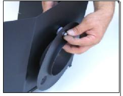
**4.** Assemble the Airaid Filter Adaptor plate using the supplied ¼ inch bolts, washers, spacers and nuts provided as shown above.
