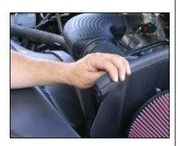
12. Install the supplied weather strip on the top edge of the Airaid Cool Air Dam. Note: The weather strip is pre cut to the proper length. Start from one end and work your way around to the other end to insure even placement.
