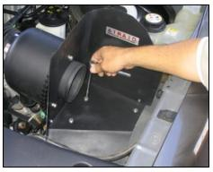
10. Finish mounting the Airaid Cool Air Dam assembly to body using the supplied ¼" nuts, bolts, washers and long bracket as shown. Note: The long bracket must be mounted under the factory mounting plate and grommets.
