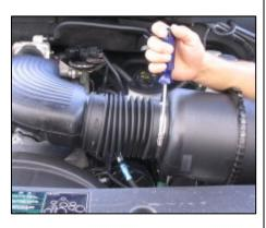
**15.** Loosen hose clamps connecting the factory intake tube to the air filter assembly and throttle body.
