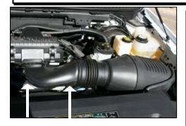
1. Disconnect negative battery cable. Grasp intake tube and sharply lift up and away from airbox
