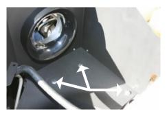
10. Mount the Airaid Cool Air Dam assembly to the vehicle using the supplied metric bolts and washers. The bolt on the right goes into the factory threaded hole. The two bolts on the left go thru the CAD, the grommets, and then the supplied bracket, with the nuts on the bottom. (Note: The mounting bracket must be on the bottom of the grommets.)
