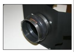
**11.** Install the hump hose and two #64 hose clamps. (*Leave loose until final adjustments are made.*)
