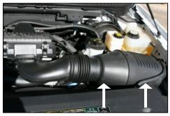
2. Grasp large oval section of intake tube and pull up and away from inner fender well, and remove entire intake tube. (Note: Intake tube is held in with rubber grommets, no bolts.)
