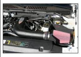
**16.** Install the Airaid air cleaner inside the cold air dam.
