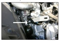
3. Remove 13mm nut on power steering reservoir bracket. Install Airaid intake tube support bracket, replace nut, and leave slightly loose. (Nut will be tightened after final adjustments.)
