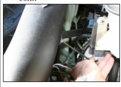
**14.** Install a 1/4x20 Allen bolt and flat washer thru the bracket at the back of the tube, and tighten. Tighten the nut at the bottom of the bracket. Tighten the hose clamps on the hump hose.
