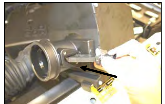
9. Reinstall the factory MAF sensor removed in step #6, into the Airaid MAF adapter as shown using two 8-32 button head screws provided in the kit. Do Not Use The Factory Screws!!
