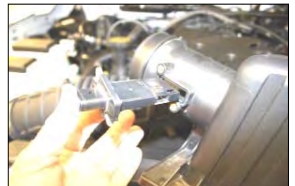
6. Using the supplied #20 Torx bit, remove two screws, and remove the Mass Air Flow sensor from the factory air cleaner lid. Save the MAF sensor for later use in step #9.
