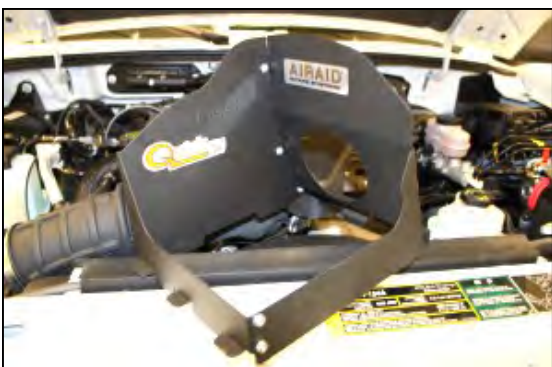
7. Assemble the two Quick Fit Panels (#2&3), using five 6-32 screws (#9), #6 flat washers (#10), and nuts (#11), as shown.
