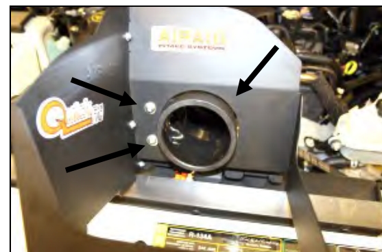
8. Install the MAF adapter (#4) into the Quick Fit Panels, using two 1/4" button head bolts (#6), and 1/4" flat washers (#7).
