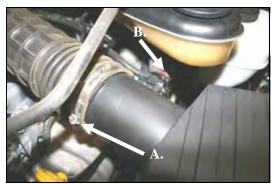
**1. Disconnect the negative battery cable! A.**) Loosen the hose clamp on the factory intake tube.
