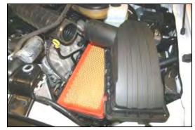
**3.** Remove the airbox lid and air filter from the vehicle.
