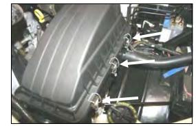
**2.** Unlatch the three metal clips that hold the airbox lid to the base.
