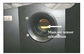
**10.** Install the MAF adapter (#4) into the panel, using four 1/4-20 button head bolts (#6), and 1/4" washers (#7). Be sure to orient the tube with the mass air sensor to the rear of the vehicle. Using a 5/32" allen wrench, tighten the 4 bolts securely.
