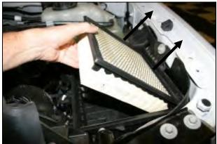
**3.** Remove the factory air filter from the airbox base.
