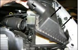
**2.** Remove the factory airbox lid from the vehicle by sliding the flexible tube off of the airbox lid neck, and then rotate the lid up and out of the base.
