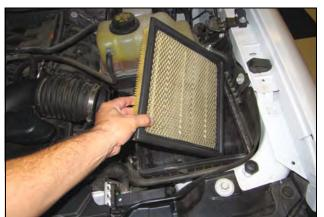
**4.** Remove the Factory air filter.
