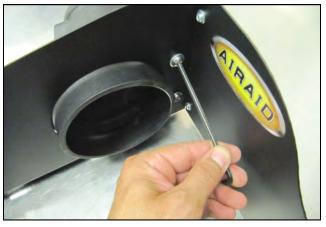
**9.** Install the Air Meter Tube (#2) into the Panel Assembly and secure using the two 1/4-20 Button Head Screws (#6),and 1/4" Flat Washers (#10).
