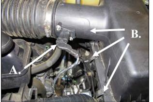
**2. A.** Disconnect the Air meter in the factory airbox top.
