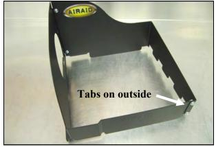
**5.** Assemble the Front and Rear Panels (# 3 & #4) as shown with the tabs on the outside of the assembly. Use the four 6-32 Button Head Screws (#9), #6 Flat Washers (#12), and #6 Kep Nuts (#11) to secure the assembly.
