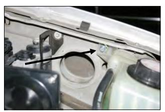
**4.** Using a 10mm socket, remove and save the 6mm bolt that secures the radiator overflow tank to the driver's side inner fender.
