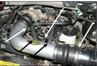
2.A). Disconnect the temperature sensor wiring harness from intake air temperature sensor.
