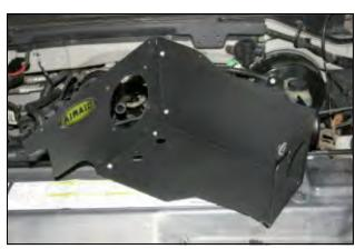
**6.** Assemble the two panels (#1) & (#2) as shown using four 6-32x3/8" Phillips head screws (#5), #6 flat washers (#6), and Kep nuts (#7).
