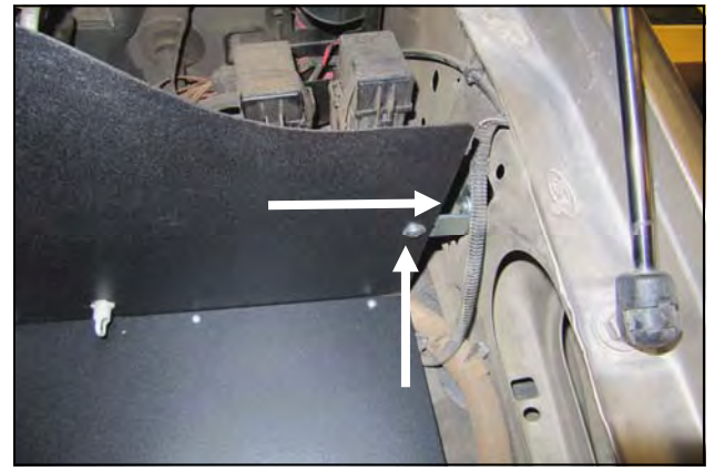
12. Vehicles equipped with a power distribution box mounted on the left inner fender, will remove the bolt from the factory bracket, slide in the bracket 140 (#12) and replace the factory bolt. If you don't have the distribution box, install the provided 1/4-20 button head bolt (#14), washer (#15), and nut (#16), through the inner fender, and tighten. Now tighten the button head bolt that holds the L-bracket to the panel.
