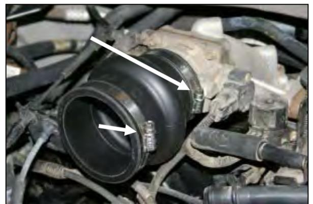
**12.** Install the small end of the reducing hump hose (#8) onto the throttlebody and tighten the #52 hose clamp (#20). Next, install the remaining #60 hose clamp (#21) on the large end of the hump hose leaving it loose for now.
