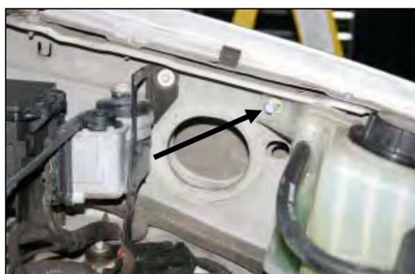
8. Using a 10mm socket, remove and save the bolt that secures the radiator overflow tank to the driver side inner fender well.
