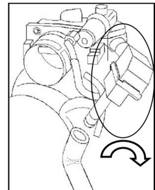
**15. 4.6L engines:** Rotate the resonator box 90 degrees to provide clearance for the 3/4 x 12" L-hose (#7). Install the 3/4"x12" L-hose (#10) onto the Airaid Intake tube and the resonator box and secure it using the two #22 speed clamps (#23).
