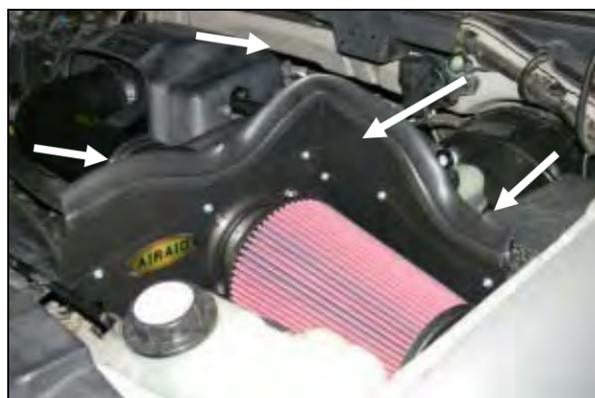
**17.** If your vehicle does not have a hood mat install the optional CAD height extender (#5) using five 6-32 screws (#12), flat washers (#13), and keps nuts (#14) as shown. Install the weatherstrip (#11) onto the top of the CAD as shown.
