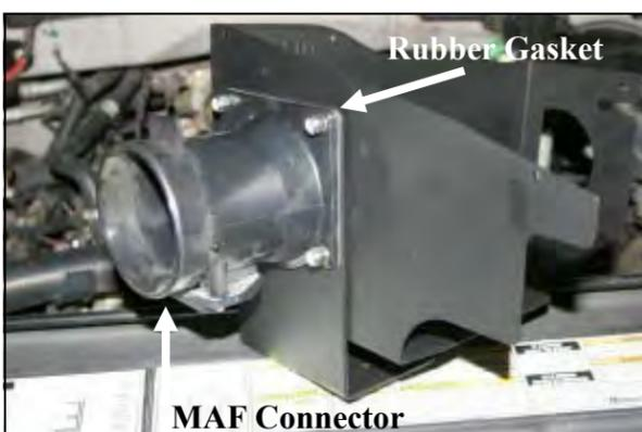
7. Attach the MAF bracket (#6), rubber gasket (#18), and factory MAF sensor housing to the Cold Air Dam (CAD) using four 1/4-20x7/8" hex bolts (#15), and 1/4" Nylock nuts (#17), as shown. Make sure that the MAF sensor connector is on the bottom when assembly is complete. Refer to the line drawing above for reference.
