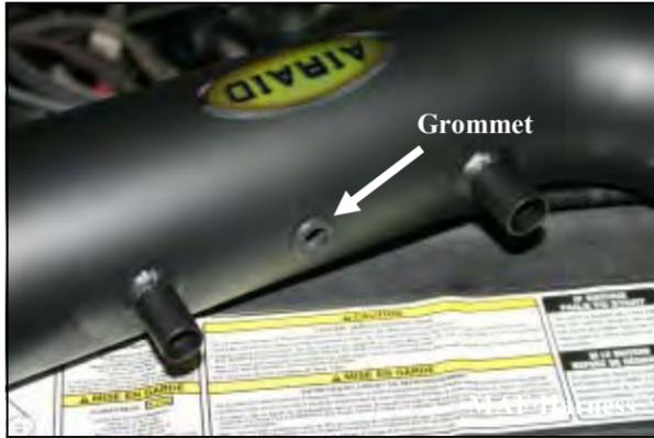
**13.** Install the supplied rubber grommet (#24) into the Airaid Intake Tube (#2) as shown.
