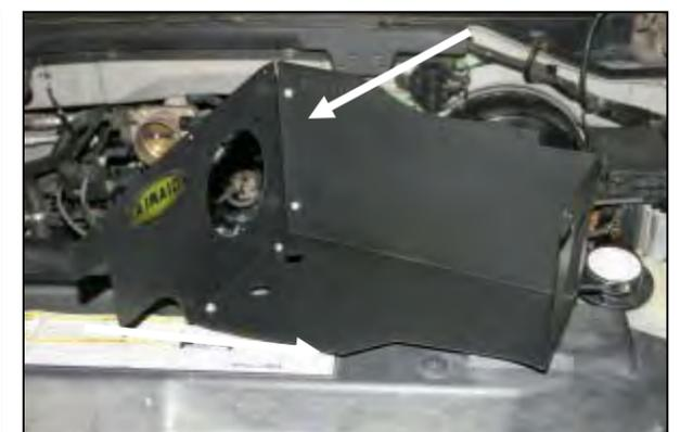
6. Assemble the MAF panel (#3), and bottom panel (#4) as shown using four 6-32 screws (#12), four flat washers (#13), and four Kep nuts (#14) as shown.
