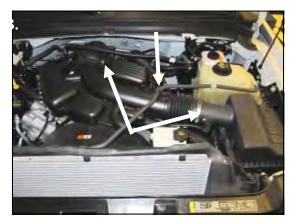
1. Disconnect the negative battery cable! Loosen the two intake clamps, unclip the coolant hose and remove the Factory intake tube.
