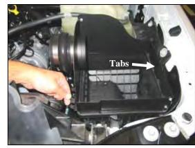
6. Install the assembly onto the lower half of the factory airbox. Slide the metal tabs into the airbox slots, and fasted the 3 airbox clips.
