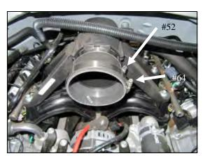
7. Install the Silicone Coupler (#5), one #64 Hose Clamp(#14), and the #52 Hose clamp (#13) onto the engine air inlet. Leave the clamps loose for now.
