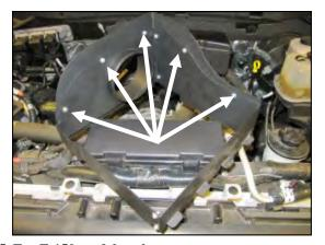
5. For F-150 models only: Fasten the Extension panel (#5) to the outside of the panel assembly using the remaining 6-32 screws, flat washers, and kep nuts.
