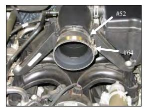
7. Install the Silicone Coupler (#6), one #64 Hose Clamp(#14), and the #52 Hose clamp (#13) onto the engine air inlet. Leave the clamps loose for now.
