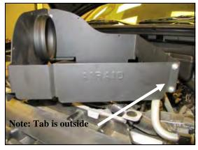
4. Assemble the two Quick Fit panels (#3 & #4) as shown using four 6-32 screws (#9) flat washers (#11) and kep nuts (#10).
