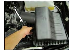
2. A.) Disconnect the Mass Air Flow (MAF) Sensor.
