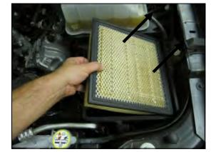
3. Remove the factory air filter from the lower half of the airbox.
