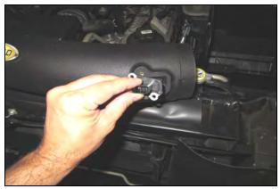
**6..** Transfer the **MAF** sensor into the Airaid Intake Tube (#2) and secure using two 8-32 x 1/2" button head screws (#10). **Do Not Use The Factory Torx Head Screws**
