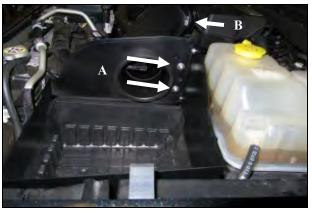
**8. A.)** Mount the Intake Tube to the Rear Panel using the two 1/4-20 Button Head Bolts (#11) and 1/4" Flat washers (#12).
