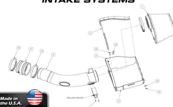
**1. Disconnect the negative battery cable!**Loosen the two intake clamps, unclip the coolant line, and remove the Factory intake tube.
