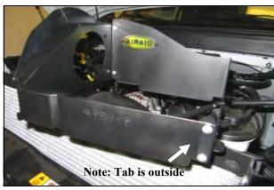
**4.** Assemble the two Quick Fit panels (#3 & #4) as shown using four 6-32 screws (#7) flat washers (#9) and kep nuts (#8).
