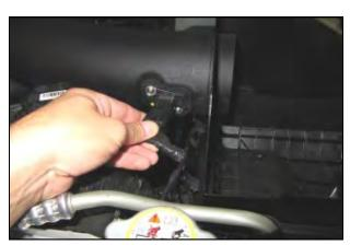
**9.** Re connect the Mass Air Flow Sensor.
