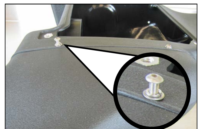
9. Secure the Scoop to the Air Box using the two sets of 8-32 Button Head Screws, Lock Washers and Flat washers.
