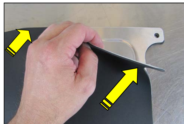
20. Remove the protective film from the top of the Air Box Lid. Prepare the underside for the Lid Gasket by cleaning it using a prep-sol or equivalent. Carefully apply the self adhesive Gasket onto the Lid as shown.
