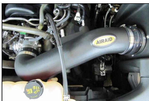
17. Insert the Airaid Intake Tube into the throttle body coupler, then into the Air box Hump Hose. Rotate the Tube forwards and backwards until proper alignment is achieved and tighten all four Clamps.
