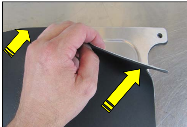
19. Remove the protective film from the top of the Air Box Lid. Prepare the underside for the Lid Gasket by cleaning it using a prep-sol or equivalent. Carefully apply the self adhesive Gasket onto the Lid as shown.
