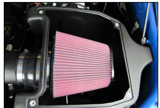
18. Install the Airaid Premium Filter onto the Filter Adapter and tighten the Clamp.
