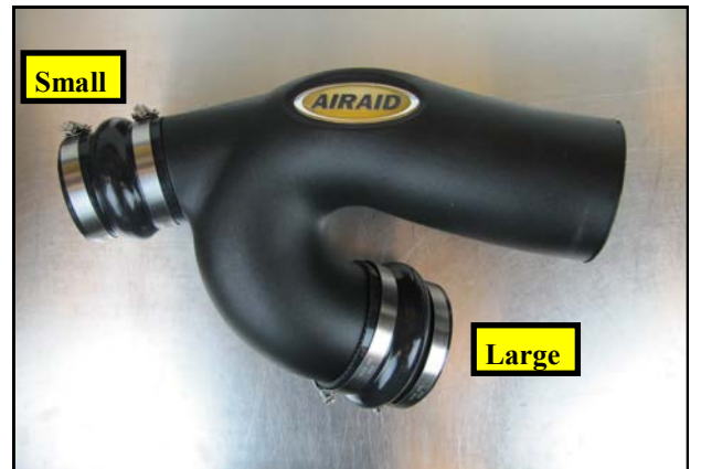
15. Slide the Hump Hoses and Clamps onto the Airaid Intake tube as shown. The Small Hump Hose will use the #48 Clamps and the Large Hump Hose is to use the #64 Clamps.
