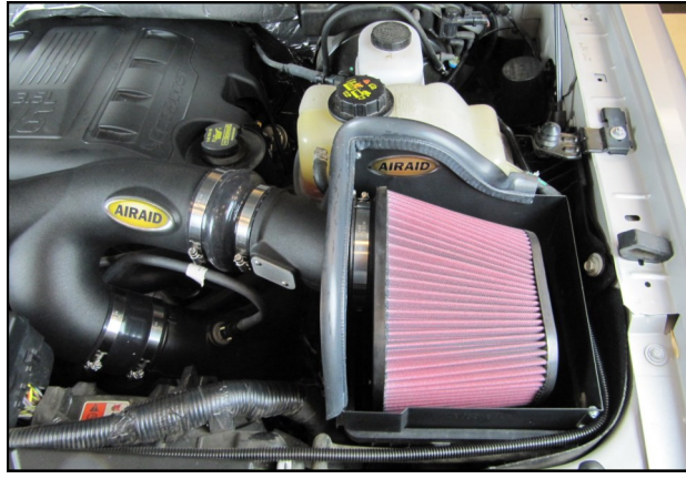
14. Install the Airaid Premium Filter onto the Sensor Tube and tighten the clamp.
