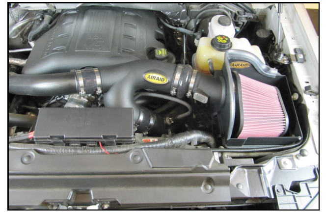
15. Double check your work. Make sure there is no foreign material in the intake path. Make sure all clamps, hoses, bolts, and screws are tight. Double check the hood clearance. Reconnect the negative battery cable.
