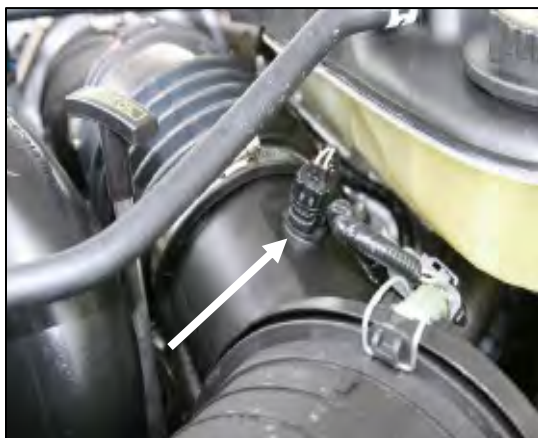
5. STOP AND LOOK! If you have a temperature sensor like this, disconnect the temperature sensor wiring harness, remove the sensor from the tube (save it for reuse) and proceed to step #8. The early production 2005 F-250 and F-350 6.0 diesel trucks either came with a temperature sensor, or they came with a Mass Air Flow (MAF) sensor. These pictures will help you determine which sensor you have. Whichever sensor you have, this Airaid Intake System will fit.
