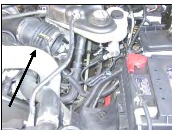
7. Remove the factory intake tube assembly. (Note: do not remove the factory flexible turbo inlet hose from the turbo housing.)
