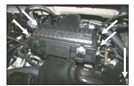
**2.** Using a 10mm deep socket, remove the 4 tower bolts, two on each side of the factory airbox. Remove one bolt holding the factory intake tube to the mounting bracket. Remove the complete factory intake system.
