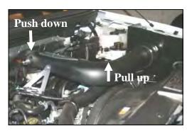
15. While gently lifting on the tube next to the radiator, and pushing down on the tube over the throttle body, tighten the two button head bolts on top of the mounting brackets. This will help make sure the Airaid Intake Tube is sealing on the throttle body.
