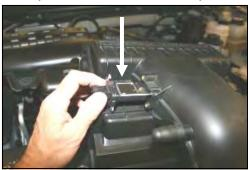
**4.** Using the provided T-20 Security Bit, remove the two screws, and remove the **MAF** sensor from the factory intake tube. Save the sensor for re-installation in the next step.
