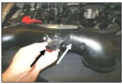
**5.** Re-install the **MAF** sensor into the Airaid Intake Tube (#5) using two 8-32 x 3/8" button head screws (#10). **Do not over tighten! Do Not Use The Factory Screws!!**
