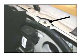
**18.** Slip the black plastic hose mount (#26) over the radiator overflow hose. Next, place one ½" flat washer (#15) over the hole on the inner drivers side fender. Slide the hose mount prongs thru the fender and thru the washer.
