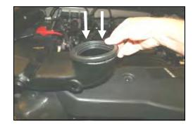
**6.** Re-install the rubber seal removed in step #3 onto the Airaid Intake Tube. Use caution to align the notch in the tube with the notch in the seal.
