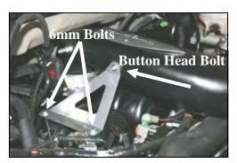
**14.** Install the two brackets (#7, #8) from the Airaid Intake tube onto the intake manifold using two  $\frac{1}{4}$  -20 x  $\frac{1}{2}$ " button head bolts (#14), and  $\frac{1}{4}$ " flat washers (#15) on the tube, and four 6mm bolts (#16), and  $\frac{1}{4}$ " flat washers (#15) on the bottom. Leave the button head bolts loose for now.
