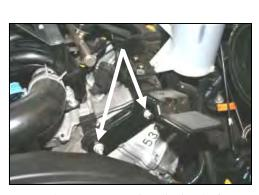
17. Factory tolerances may require adjusting the factory bracket to align the tube and hump hose with the filter adapter. Therefore, it may be necessary to loosen the two mounting nuts with a 13mm deep socket, and adjust it.
