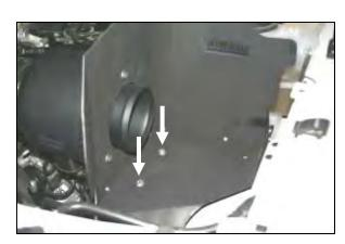
12. Insert two  $\frac{1}{4}$ -20 x  $\frac{7}{8}$ " bolts (#9) and  $\frac{1}{4}$ " flat washers (#10) through the holes in the CAD and thru the grommets. On the underside of the factory airbox mounting plate, align the long/narrow bracket (#16), two  $\frac{1}{4}$ " flat washers (#10), and two  $\frac{1}{4}$ -20 nuts (#12) with the  $\frac{1}{4}$ -20 x  $\frac{7}{8}$ " bolts. Tighten the assembly securely.
