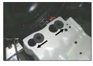
**9.** Slip two rubber grommets (#14) into the large holes in the factory airbox mounting plate, and then slide them sideways into the small holes as shown.
