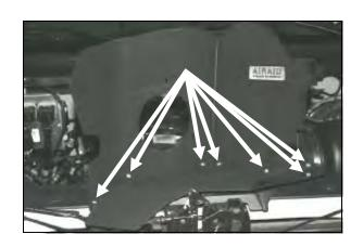
**4.** Assemble the Airaid Cool Air Dam (CAD) panels (#2, #3) using seven 6-32 x 5/16" screws (#6), #6 flat washers (#7), and 6-32 keps nuts (#8).
