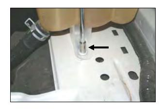
**3.** Using a 5/16" socket, ratchet and extension, remove one bolt from the factory coolant reservoir mount.
