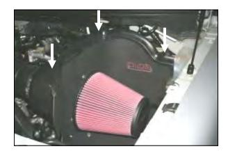
**14.** Install the weather strip (#5) onto the top edge of the **CAD** as shown. (*Hint: start at one end and work your way around to the other.*)
