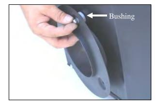
**5.** Insert three ½-20 x 7/8" bolts (#9), and ½" flat washers (#10) through the CAD. Place one bushing (#11) at each hole between the **CAD** and the filter adapter (#4). Next, secure the assembly using three 1/4" flat washers (#10), and 1/4-20 nuts (#12).
