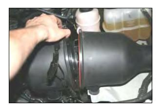
1. Disconnect the negative battery cable. Unclip the factory airbox from the factory Mass Air Flow (MAF) sensor housing.
