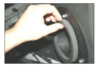
6. Install the supplied gasket (#13) onto the filter adapter.
