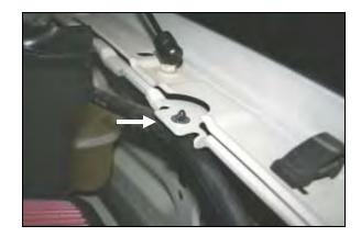
**15.** Slip the black plastic hose mount (#17) over the radiator overflow hose. Next, place one ½" flat washer (#10) over the hole on the inner drivers side fender. Slide the hose mount prongs thru the fender and thru the washer.
