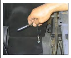
9. Mount the Airaid Cool Air Dam assembly to the vehicle using the supplied metric bolt and washer and the factory bolt hole as shown above.
