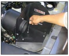
10. Finish mounting the Airaid Cool Air Dam assembly to body using the supplied <sup>1</sup>/<sub>4</sub>" nuts, bolts, washers and long bracket as shown. *Note: The long bracket must be mounted under the factory mounting plate and grommets.*
