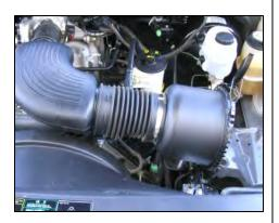
**2.** Remove air filter and air box from vehicle.
