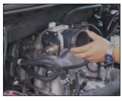
18. Install supplied silicone reducer on end of throttle body. Install #48 hose clamp on small end of the reducer and #56 hose clamp on the big end of the reducer. Leave hose clamps loose until final assembly.
