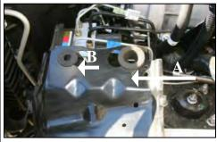
**6.** *A.*) Remove the two factory grommets by sliding sideways. *B.*) Install the two supplied grommets in reverse order.
