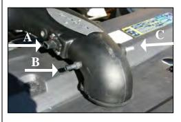
8. Remove the mass air sensor from the stock airbox using the #20 torx tool. *A.*) Using the supplied 8/32 screws install the mass air sensor in the Airaid intake tube. *B.*) Install the 3/8" plastic hose fitting. **Do not over tighten!** *C.*) Install the supplied grommet, and then the supplied aluminum fitting, rounded end first.
