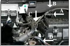
**4.** *A.*) Remove breather line by pushing up on green lever and pulling fitting away from airbox. *B.*) Remove vacuum line from clip. *C.*) Pull up on, and remove heater control valve from tower bolt. *D.*) Pull up on, and remove wiring harness from tower bolt.
