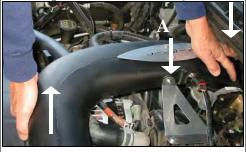
over the throttle body, and into the hump hose. A.) Install the two ½-20 Allen bolts and washers thru the brackets and into the tube. Push down on the throttle body end, and lift up on the curve of the tube.
