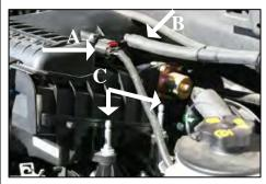
5. *A.*) Unhook the mass air flow sensor by pulling out the red plastic tab first, and then remove the plug. *B.*) Unhook the vacuum line. *C.*) Remove all four tower bolts and remove air box. (Save tower bolts for reinstallation.)
