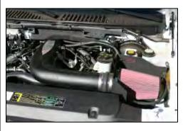
**16.** Install the Airaid Premium Filter inside the cold air dam.
