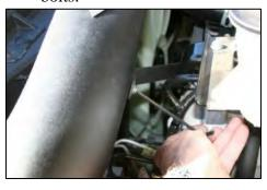
14. Install a ¼-20 Allen bolt and flat washer thru the bracket at the back of the tube, and tighten. Tighten the nut at the bottom of the bracket. Tighten the hose clamps on the hump hose.
