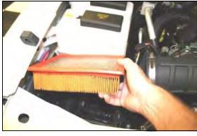
**5.** Remove the factory air filter from the factory air cleaner base.
