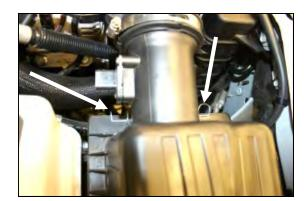
**3.** Unlatch the two metal clips that hold the factory air cleaner lid to the base.
