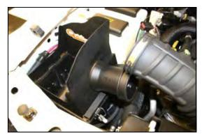
**10.** Install the Quick Fit Assembly onto the top of the factory air cleaner base. Start by sliding the three tabs on the Airaid panel thru the three slots on the top of the base. Center the panel assembly, and re-latch the two factory clips.
