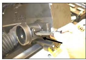
**9.** Reinstall the factory **MAF** sensor removed in step #6, into the Airaid **MAF** adapter as shown using two 8-32 button head screws provided in the kit. **Do Not Use The Factory Screws!!**
