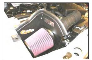
**13.** Install the Airaid Premium Filter (#1) into the **MAF** adapter, and tighten the hose clamp. Next install the weather strip (#5) onto the top of the Quick Fit Panels as shown.
