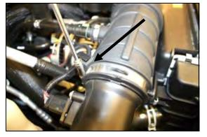
1. <u>Disconnect the negative battery cable.</u> Loosen the hose clamp that holds the factory intake tube to the air cleaner lid.
