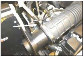
**11.** Reconnect the factory intake tube to the Airaid **MAF** adapter, and then tighten the hose clamp.
