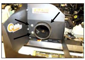
**8.** Install the **MAF** adapter (#4) into the Quick Fit Panels, using two 1/4" button head bolts (#6), and 1/4" flat washers (#7).
