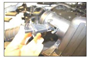
**6.** Using the supplied #20 Torx bit, remove two screws, and remove the Mass Air Flow sensor from the factory air cleaner lid. Save the MAF sensor for later use in step #9.
