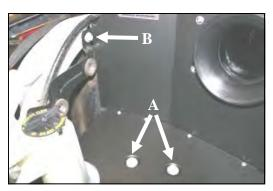
**11. A.**) Align the two panel holes with the air cleaner base support holes on the vehicle. **B.**) Align the tab on the panel with the radiator support bolt hole. The tab will mount on top of the bracket.
