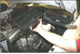
**4.** Remove the base assembly by pulling it up out of the mounting grommets. Using the supplied torx bit (#14), 1/4" socket, ratchet and extension remove the two screws holding the factory mass air sensor in place, and remove the mass air sensor from the air cleaner lid.
