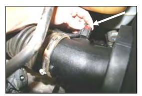
**13.** Reconnect the factory air intake tube onto the MAF adapter (#4), and tighten the hose clamp securely. Next, re-connect the mass air flow sensor wiring harness onto the sensor.
