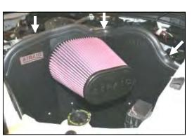
**14.** Install the Airaid Premium Filter (#1) onto the MAF adapter and tighten the clamp. Next, install the weather strip (#5) onto the top of the CAD, starting next to the fender and working your way towards the radiator.
