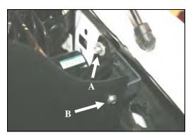
12. A.) Slide the L-bracket under the antilock braking system bracket, and re-install the bolt removed in step #8.B.) Fasten the bracket onto the back of the
