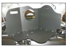
**9.** Assemble the two Cool Air Dam panels (#2 and #3) as shown, using seven 6-32 screws (#10), #6 washers (#11), and keps nuts (#12). Tighten securely.
