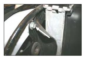
**7.** Using a 1/2" socket, ratchet, and extension, remove one bolt attaching the air cleaner base alignment bracket to the radiator support. The bolt will be reused in step #11.
