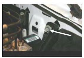
**8.** Using a 10mm socket, remove one bolt which secures the anti lock braking system bracket to the drivers side inner fender. The bolt will be reused in step #12.
