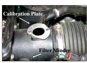
**9.** *A.*) Install the Calibration Plate onto the Cool Air Box using two 8-32 x 1/2" Flat Head Screws (#15). **B.**) Reinstall the factory grommet, and filter minder into the Cool Air Box, and then reconnect the filter minder wiring harness.
