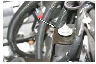
3. Remove one bolt from the factory airbox mounting plate, and save it for reinstallation in step #8.
