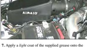
inside of the factory tube. Install the Airaid Cool Air Box into the vehicle making sure it is seated correctly into the factory grommets, and the inlet is aligned with the factory hole in the fender. Slide the factory intake tube over the O-ring and then tighten the factory hose clamp.
