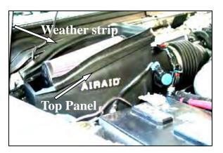
11. Install the Airaid Premium Filter (#1) onto the filter adapter, and tighten the hose clamp. Next install the Top Panel (#3) onto the top of the Cool Air Box using six 8-32x3/8" button head bolts (#10), and #8 flat washers (#11). Install the weather strip (#5) onto the edge of the top panel as shown
