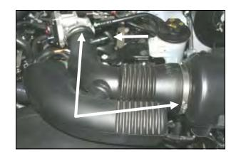
**3.** Slide the green tab on the factory breather hose, and remove it from the factory intake tube. Using a 5/16" socket, loosen the hose clamps on each end of the factory intake tube and remove it from the engine.
