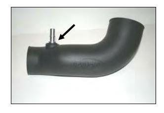
**8.** Install the rubber grommet (#22), and aluminum fitting (#21) into the Airaid Intake Tube (#4).
