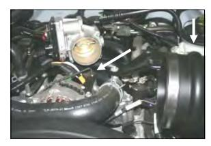
**14.** Using a 10mm socket, remove one factory bolt from under the throttle body. Using a 5/32" allen wrench, install the M6x1x20 button head bolt (#26) in its place. Install the urethane hump hose (#6) and two #80 hose clamps (#25) onto the factory **MAF** sensor housing. (Leave the clamps loose for now).
