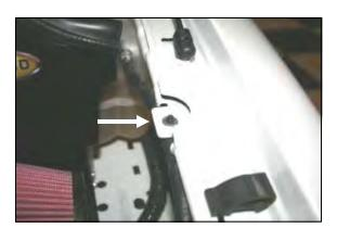
17. Slip the black plastic hose mount (#20) over the radiator overflow hose. Next, place one ½" flat washer (#13) over the hole on the inner drivers side fender. Slide the hose mount prongs thru the fender and thru the washer.
