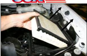
**3.** Remove the factory air filter from the airbox base.
