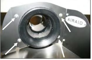
6. Install the Quick Fit Assembly onto the top of the factory airbox base sliding the four tabs on the panel into the slots on the base and then latching the three factory latches. Slide the factory intake tube over the MAF tube and tighten the factory hose clamp as
