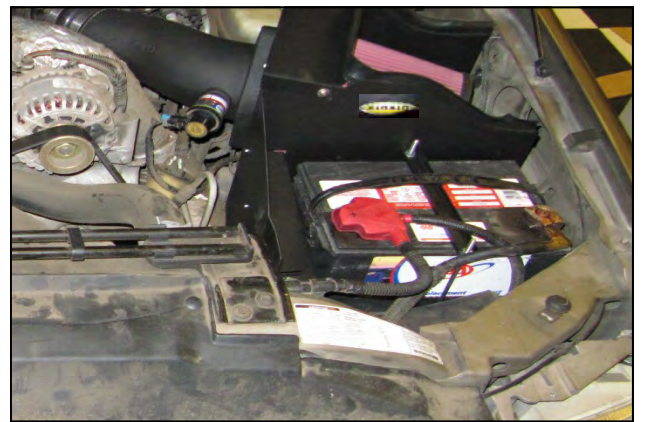
18. Double check your work! Make sure there is no foreign material in the intake path. Make sure all clamps, hoses, bolts, and screws are tight. Double check the hood clearance. Reconnect the battery cables.
