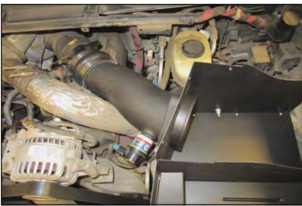
10. Insert the Airaid Intake Tube into the CAD assembly, then slide the Hump Hose onto the turbo inlet and tighten the Clamps. Reconnect the filter minder.
