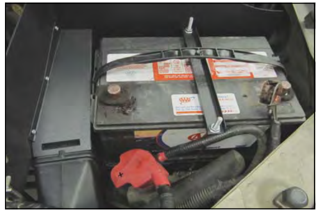
15. Secure the battery in place using the new 1/4-20 J Bolts(#11), Tie Down (#8) and 1/4-20 Flange nuts. The CAD Panels are slotted to accommodate the J Bolts.
