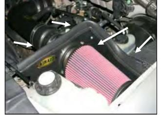
**16.** Reinstall the beauty cover using the 3 factory bolts. Install the Airaid Premium Filter (#1) as shown, and tighten the hose clamp.
