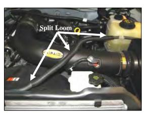
**9. A.)** Insert the Airaid Intake Tube into the couplers as shown. Check for alignment, and tighten all clamps. **B.**) Slide the Split Loom (#8) over the coolant line **C.**) Re connect the Mass Air Flow Sensor.
