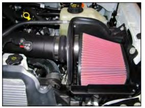
**10.** Install the Airaid Premium Filter (#1) to the mounting flange inside the quick fit assembly. Complete the installation by attaching the Weather Strip (#7) to the top of the panels as shown.
