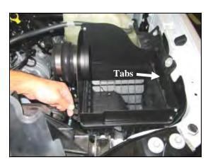
6. Install the assembly onto the lower half of the factory airbox. Slide the metal tabs into the airbox slots, and fasted the 3 airbox clips.
