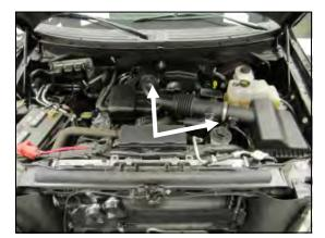
1. Disconnect the negative battery cable! Loosen the two intake clamps and remove the Factory intake tube.
