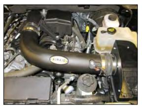
9. A.) Insert the Airaid Intake Tube into the couplers as shown. Check for alignment, and tighten all clamps. **B.**) Re connect the Mass Air Flow Sensor.
