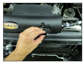
8. Transfer the MAF sensor into the Airaid Intake Tube (#2) and secure using two 8-32 x 3/8" button head screws (#11). Do Not Use The Factory Torx Head Screws !
