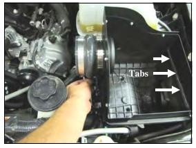
6. A.) Install the Silicone Hump Hose (#7) and two #64 Hose Clamps(#14) onto the Quick Fit assembly. Leave the clamps loose for now.
