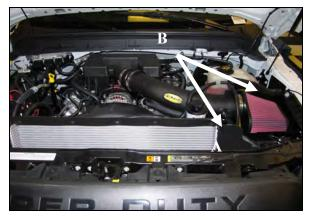
**11. A)** Install the Airaid Premium Filter (#1) to the mounting flange inside the quick fit assembly. **B)** Complete the installation by attaching the Weather Strip (#6) to the top of the panels as shown.
