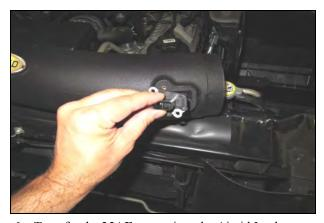
**6.** Transfer the **MAF** sensor into the Airaid Intake Tube (#2) and secure using two 8-32 x 1/2" button head screws (#10). **Do Not Use The Factory Torx Head Screws**
