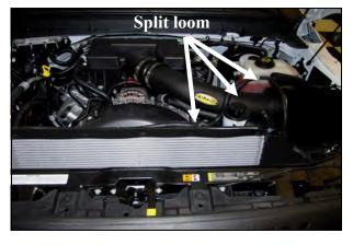
**10.** Slide the 20" section of Split Loom (#8) over the Coolant line to protect it from chaffing on the intake tube.
