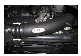
7. Install the Hump Hose (#5), and the clamps (#13) onto the Intake Tube. Slide the hump hose and clamps down the tube as far as they will go and leave the clamps loose for now.
